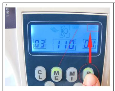
You can now start sewing the stitches (see image 8, we sew without the footcontrol). The machine stitches the three stitches and stops.
