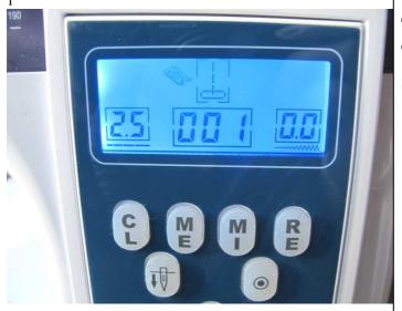
Turn on the machine. The machine shows straight stitch 001.
